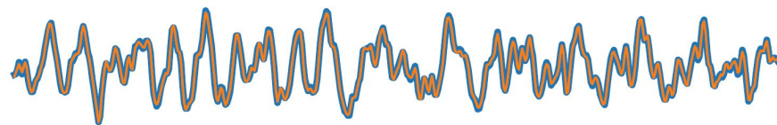
Figure 2. Original waveform (blue, thick line) with adversarial waveform (orange, thin line) overlaid; it is nearly impossible to notice a difference. The audio waveform was chosen randomly from the attacks generated and is 500 samples long.
